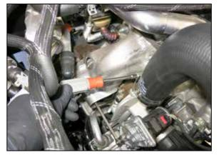
charge pipe onto the provided quick connect coupler as shown. **NOTE: Be sure to install the O-ring in the correct direction as noted in the previous step.**
