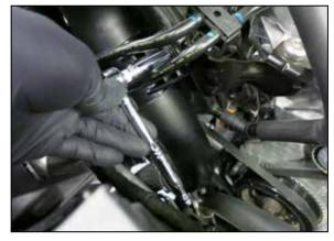
20. Remove the bolt that secures the charge tube to the mount.
