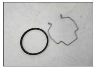
6. Remove the locking clip and O-ring from the factory charge pipe. **NOTE: Pay attention to the direction the O-ring is installed into the factory charge pipe, it will need to be installed into the supplied coupler in the same direction.**
