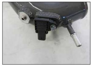
10. Remove the pressure sensor from the factory charge tube and install it into the K&N tube using the provided hardware.
