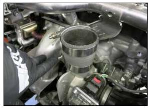
25. Install the provided step hose onto the turbo outlet and secure with the provided hose clamp.
