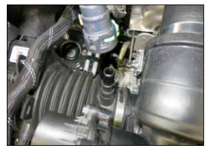
16. Release and disconnect the other end of the CCV line from intake tube.
