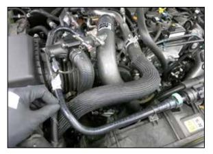
31. Reinstall the CCV hose to the quick connect fittings. Install the K&N decal as shown.
