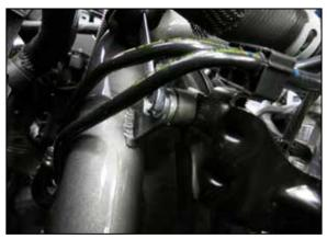
28. Insert the charge tube into the Coupler at the turbo outlet and the intercooler inlet hose, adjust the tube for best fit and then secure the hose clamps. Fully tighten the charge pipe mounting nut.
