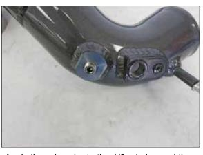
9. Apply thread sealer to the 1/8npt plug and then install the plug into the accessory port.
