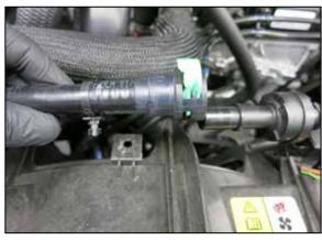
15. Release the green locking tab and then disconnect the CCV quick connect fitting and detach it from the radiator shroud.
