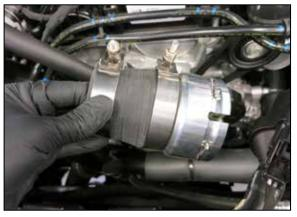
12. Install the quick connector assembly onto the inter cooler, push the assembly on until the locking clip snaps into position. **NOTE: The notch shown on the quick coupler needs to align with the index tab on the intercooler.**
