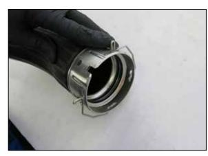
4. Release the locking clip securing the charge tube to the intercooler. Push the clip back until it snaps into the unlock position. NOTE: the charge tube is removed in picture to show the clip in the unlocked position.
