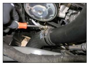
19. Loosen the hose clamp that secures the hotside charge tube to the intercooler inlet hose.
