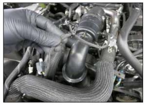
17. Disconnect the BOV electrical connection and unhook the wiring harness from the mounting post.
