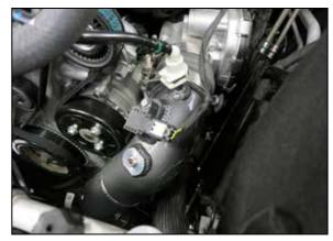
14. Connect the EVAP vent line to the quick connect fitting on the charge tube and then reconnect the pressure sensor electrical connection. This completes the cold side charge pipe installation.
