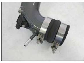
11. Install the provided hump coupler onto the K&N charge pipe and secure with the provided hose clamp.
