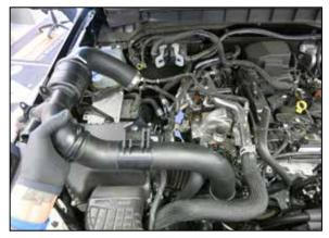
22. Remove the hot-side charge pipe from the vehicle.
