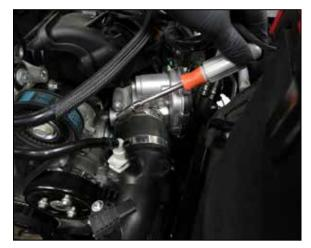
3. Loosen the hose clamp that secures the charge pipe to the throttle body.
