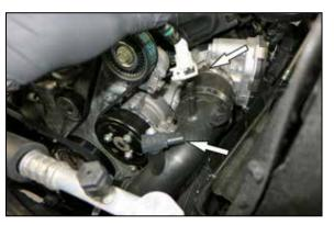
2. Remove the green locking clip and then disconnect the EVAP hose from the cold-side charge pipe. Disconnect the pressure sensor electrical connection.
