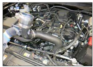
5. Pull the charge pipe back from the throttle body and unhook it from the intercooler, then remove the factory cold-side charge pipe from the vehicle.
