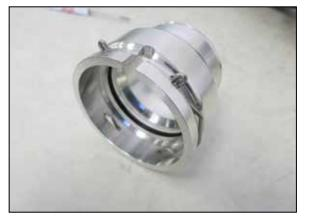
7. Install the O-ring and locking clip from the factory
